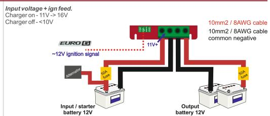
By applying a live signal to the ignition connector you put the BB into ignition dependent mode. The BB shall NOT work unless it has a live ignition signal - even if you remove the ignition feed cable and provide 13.5V+ onto the input terminal.
