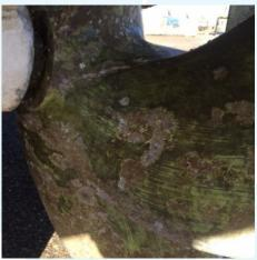
Isolated blistering and patches of Propspeed falling off are usually a clear indicator that electrolysis is occurring on the vessel.
