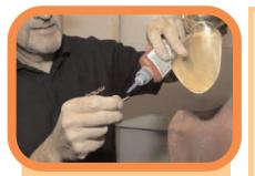
Fit the anode, applying locktite to the two screws before tightening them.
