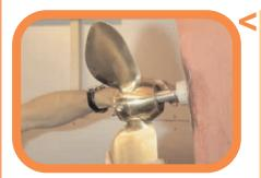
Replace the propeller on the shaft, making sure that the propeller forward hub face aligns with the pen mark. If it does, continue with step 1.6. If it does not it is because the key is too tall for the keyway in the propeller. In this case follow step 1.5
