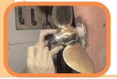
Finally, the movement of the propeller should be re-checked. It should be free from forward to reverse position, requiring only the pressure from one finger on a blade tip
