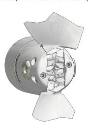
**8** Tighten both pivot pin locking screws (9) using the Allen wrench (15) supplied; If using torque wrench tighten to about 1.2 Kpm=12 Nm=8.4 ft-lb;
