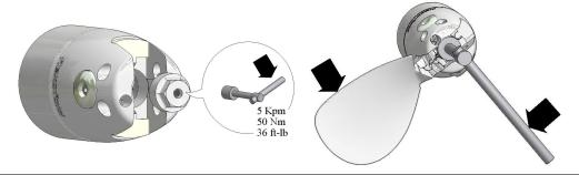
**2** Slide tab washer (5) on to shaft nut locking screw (6); screw in through hole in the shaft nut into end of shaft and tighten firmly; If using torque wrench tighten to about 0,5 Kpm=5 Nm=3.6 ft-lb;
