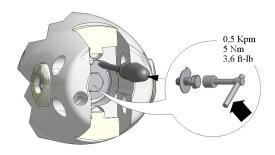
**3** Again using a straight screw driver: Bend side of tab washer up over hex on the shaft nut locking screw (6).
