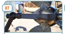
Tap end of removing tool to extract the pitch stop ensuring the blades are in the feathered position.
