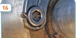
...you can then fully open legs of split pin, with a small screw driver
