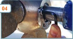
...and then remove cap screws with allen key provided.
