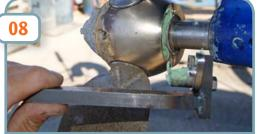
..and then remove the pitch stop from the hub. It is important that the blades stay in the feathered position until the new pitch stop has been fitted.
