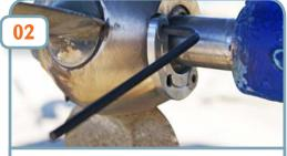
On older models you may have Counter sunk screws, remove with allen key provided.
