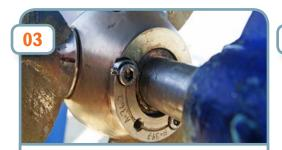
On newer models cap screws are fitted, remove split pin...
