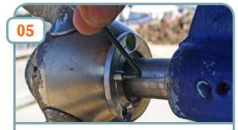
Remove centre grub screw, if fitted.
