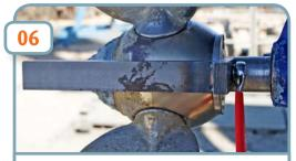
Fit removing tool into grub screw hole with bolt and washer provided.
