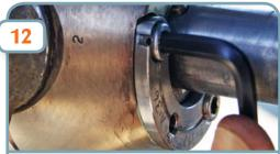
Tighten, bringing the hole in the cap screw inline with the cut-out in the pitch cassette.
