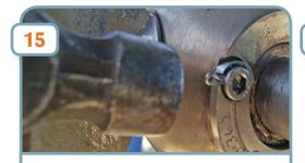
Tap end on split pin, this should encourage the legs of the pin to open...
