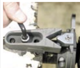
2 The fixed blade fitted here sits on a bearing which will have to be replaced every two years or so
