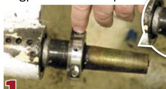
2 With the fixing point marked the shaft is drilled
