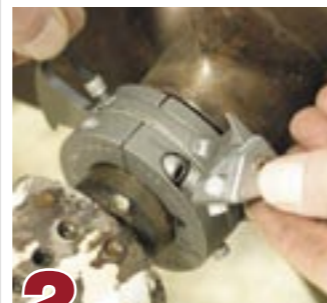
1 Coming in two parts or more, a scissor cutter can be attached without removing the prop
