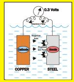
This release of small particles (ions) into the water is much more rapid than with one metal alone, and is limited to the corrosion of the steel. The cathode material (copper) is protected.
