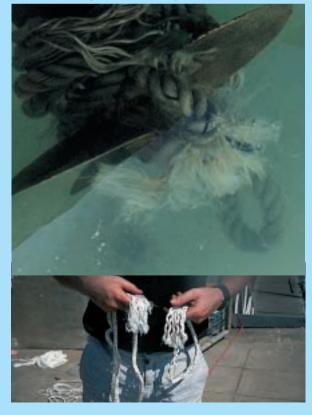
The Stripper might be the most expensive of the five cutters tested, but it also proved to be the most efficient. If you want a cutter that will see off most materials, then we would recommend this product. Although it was a close run thing between it and the Spurs, the quality of the Stripper and its ability to shred everything we chucked at it, definitely gave it the edge.
