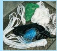
The ropes were cut into equal lengths of about 2.5m while the netting and plastic sheet was cut into 1m squares. The engine was started and run at a fast idle of around 1,200rpm. Each sample was fed into the flow of the rotating propeller. The ropes were held at one end to simulate the extra drag created when anchored to a pot, and the ability of each rope to wrap itself around the P-bracket as it was pulled into the propeller.
