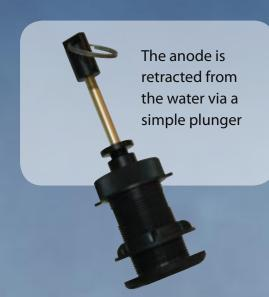
Most boat owners know the damage caused by electro - chemical reaction when metal parts are immersed in salt water without suitable protection – if they don't, they soon will! No protection can cause very expensive and potentially dangerous damage, and often in a very short space of time.
