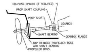
In most installations, the gap between the propeller hub and the shaft bearing is wide enough to allow the installation of a Prop Protector. This gap must be sufficiently wide to accommodate the cutter plus an additional gap of 6mm (1/4 inch) between the Protector and the bearing. Extra Large cutters need a gap of approximately 12mm (1/2 inch).
